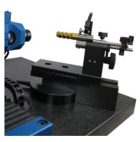
The PG concentricity fixture, also known as a 3 roller, provides a constant smooth part rotation that allows for easy and accurate measurements of the tool. All precision concentricity fixture are certified to be accurate within 2µ over the rollers. Each
